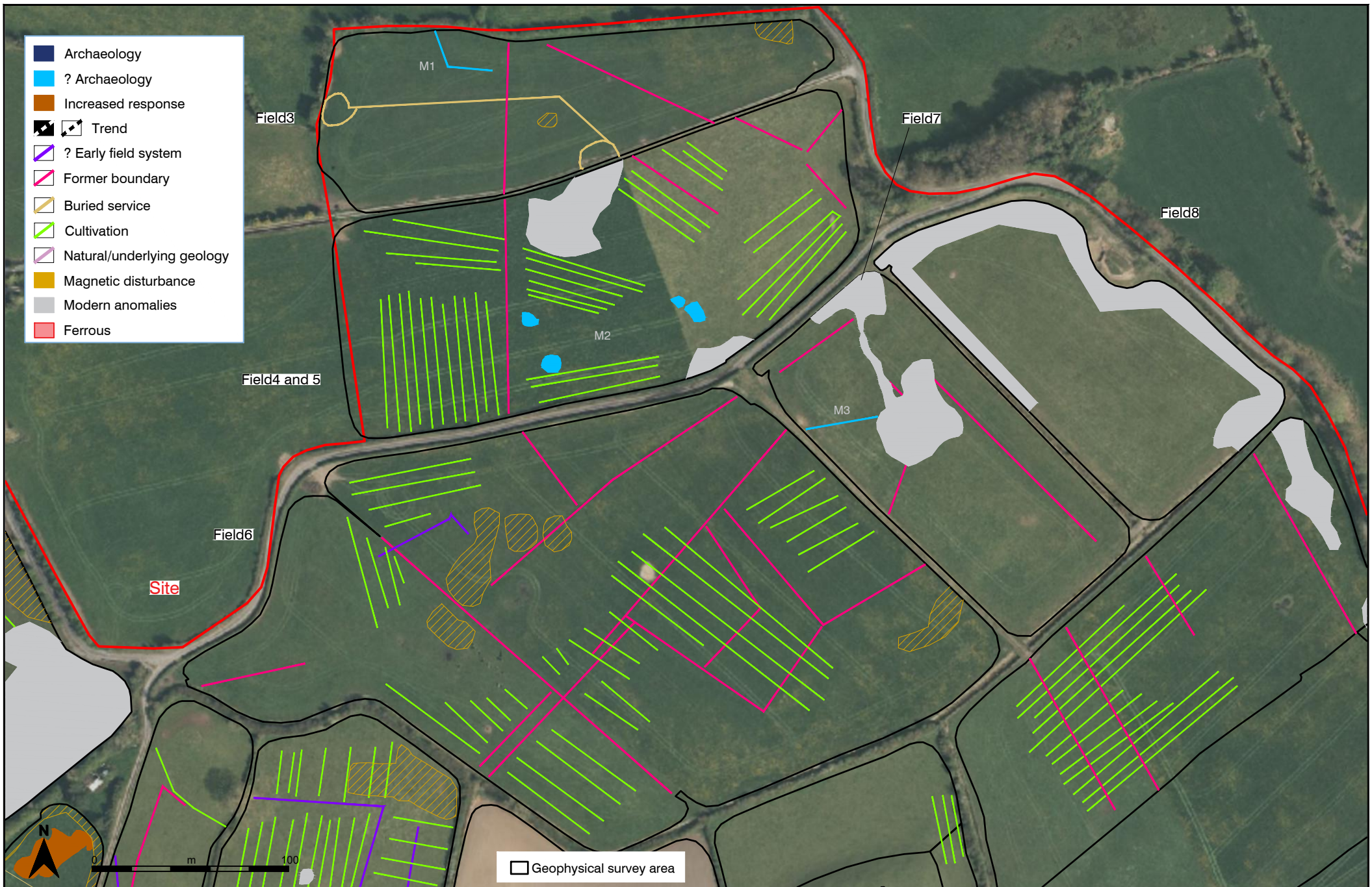
Figure 12 Aerial view of site, showing geophysical survey interpretation of fields 3 to 8
